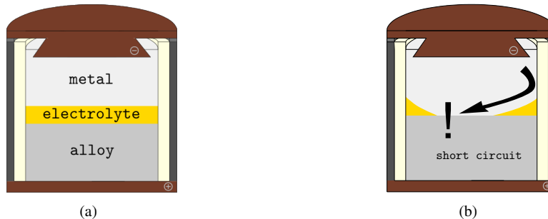
Figure 1: Sketch of a liquid metal battery with typical inventory (a) and short circuit due to strong fluid flow (b).
