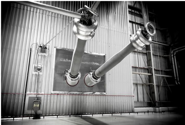
Figure 1: 600 kV HVDC transformer bushings.
